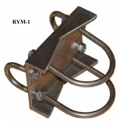
RYM-1 are used to mount Yagi antennas to vertical members 33-50 mm OD. Material – steel +Zn+Cd . Net weight 0.44 kg
